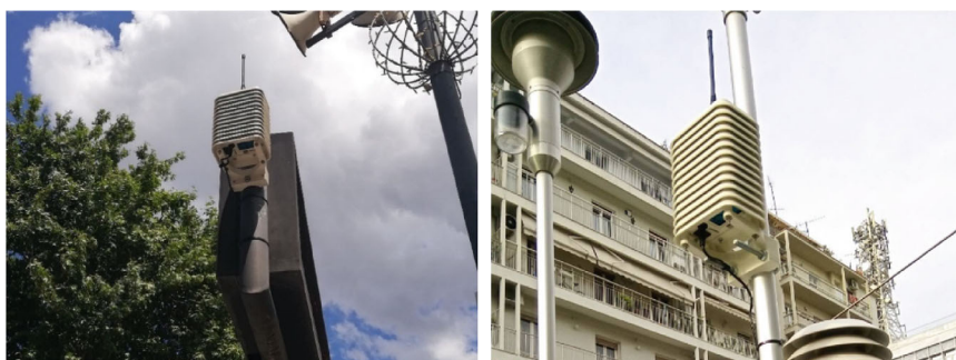
Fig. 2 Examples of installed LCAQSN nodes of the KASTOM project in the field
